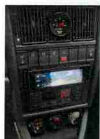
Console houses AEM AFR at top, oil pressure, oil temp and boost at bottom, with JVC head unit in center. Wood trim painted flat black
