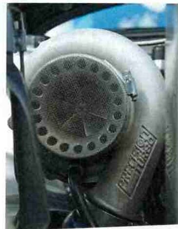
VR6 swap was the route to 516awhp, 460 lb-ft thanks to 2.9L overbore, big-valve ported head, 288° cams, Precision turbo, Kinetic manifold, 034 intake manifold and standalone, Snow water/meth injection
