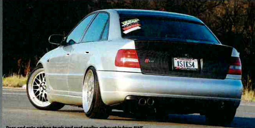
Rear-end gets carbon trunk and roof spoiler, exhaust is from AWE
