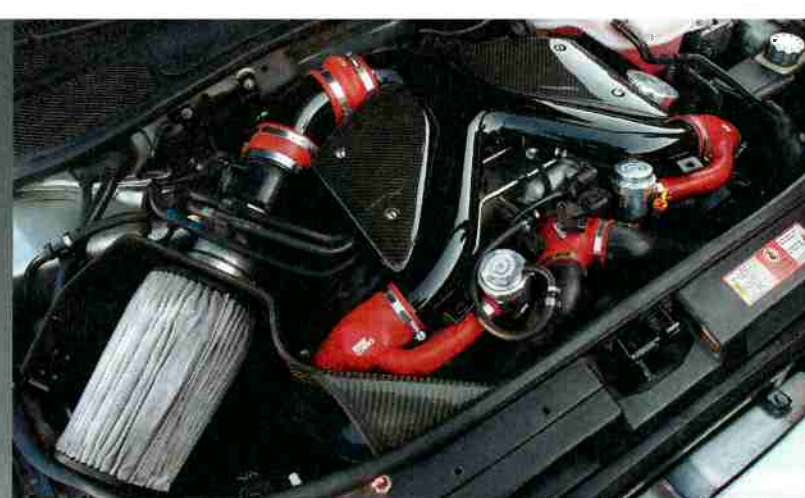
2.7L V6 has AWE stage 3 K04 turbos, GIAC software, big injectors and Induktion downpipes to produce about 430hp
